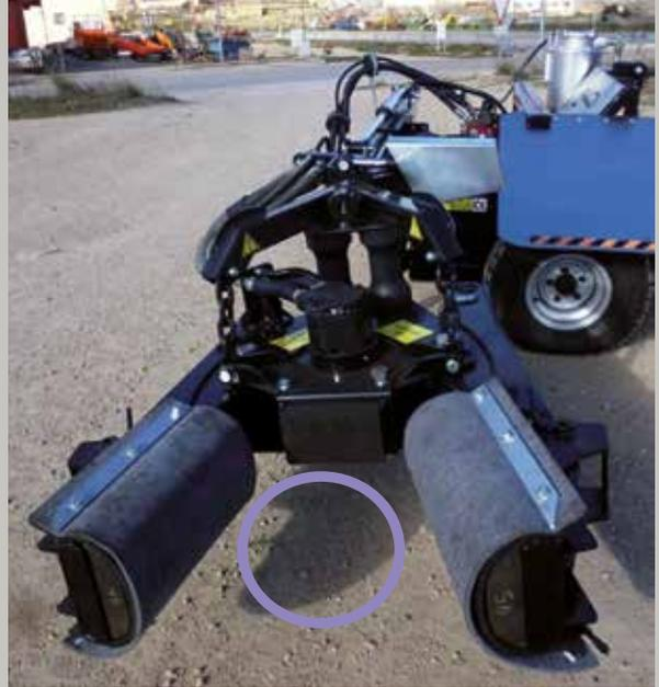
1. Place the block support and clamping cylinders in the most appropriate position according to the girth of the trees to be harvested.
